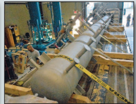
30" Dia. 8' 0" Horizontal Surge Drums with Level Columns Mounted
