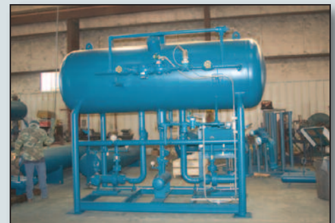
Liquid recirculator package with pumps and controls
